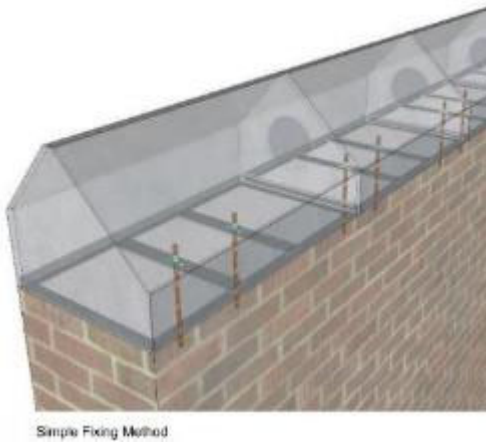
Figure 4-32 GRP Parapet Extension
